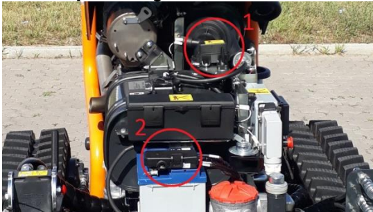
Position of "1" Main and "2" Starter Fuse Boxes
